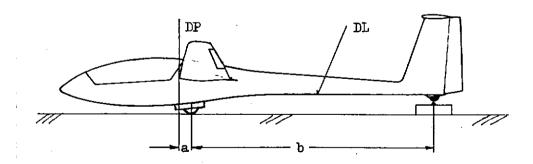
DATUM LINE (DL): under side of fuselage boom placed horizontal. DATUM POINT (DP): leading edge of wing at root.
